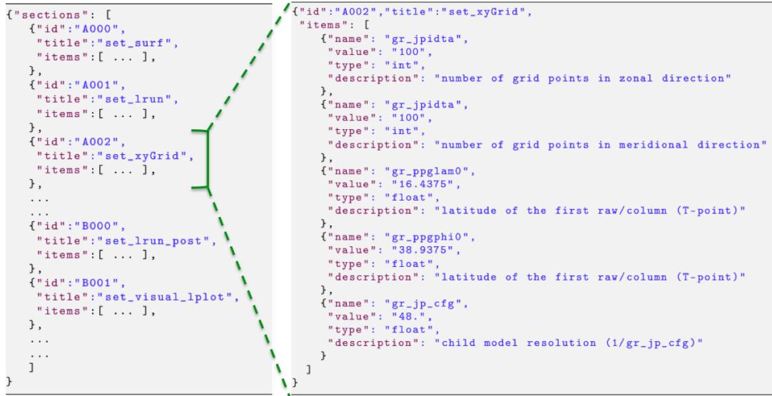
Figure 5.1. JSON representation for the SURF-NEMO user-configuration file.
